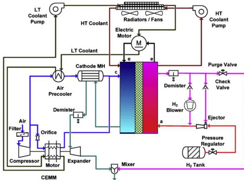
Figure 1. An automotive fuel cell system configuration
